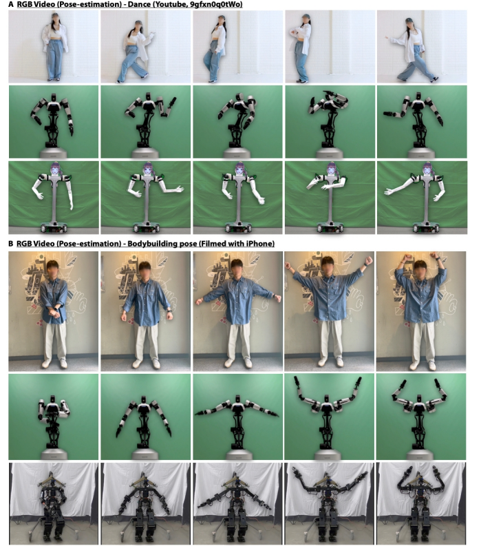
Fig. 9. Result of retargeting from estimated motion data from RGB video to robots. (A) The result of retargeting from the moving person's image to the robot with the base fixed. By considering the characteristics of the original motion, we achieved successful retargeting of AMBIDEX and JF2. (B) The result of retargeting the motion obtained from the RGB video taken with the iPhone to AMBIDEX and THORMANG.
