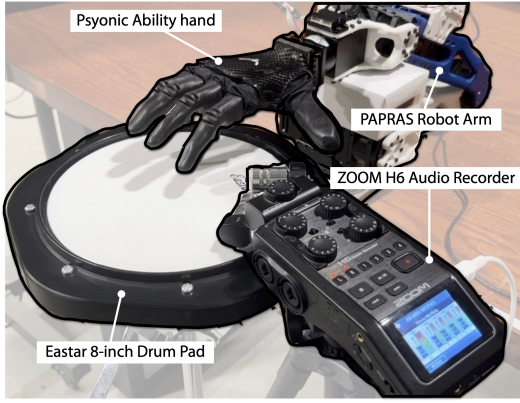
Fig. 2: The hardware setup includes PSYONIC Ability Hand, mounted on a 6-DOF PAPRAS robot arm. Sound recording is performed using a ZOOM H6 recorder. An 8-inch Eastar Drum Practice Pad is utilized as the tapping object.
